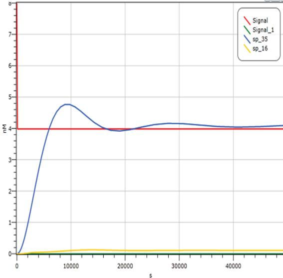
**Figure 1:** Step response of a constant gain system under a so-called PI controller; this system is explained in [2]. Output of this idealized DSD implementation using Visual DSD software ([6]) is structurally similar to the output of an *in silico* implementation of PI controller, e.g., using MATLAB, except for the fact that the time-scale is quite large. The reason why the time scale is so large is due to the fact that the DSD reactions cannot proceed arbitrarily fast.
