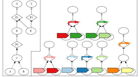
Figure 1: A regulatory DAG specification (left) and library (right) constructed from GCMs. Circles are species nodes, diamonds are promoter nodes, open arrows are production edges, closed arrows are activation edges, tee arrows are repression edges, and dotted arrows are complexation edges. Colored bent arrows and box arrows represent the different SBOL promoter and coding sequence DNA components that annotate the source GCMs for the DAG library.
