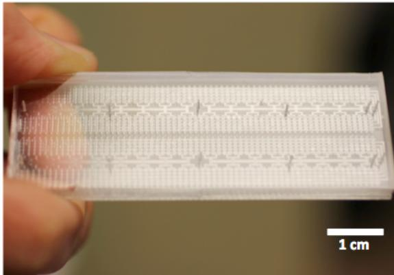
**Figure 3. Optical image of a microfluidic device designed for the parallel assembly of 256 distinct genetic circuits.**
