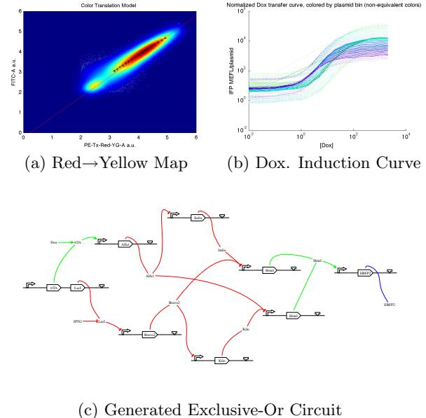
**Figure 1:** Example results from the three web services currently available on the TASBE tools site: (a) calibration of unit translation for a Color Model, (b) transfer curve (mean (solid lines) and standard deviations (dashed lines)) binned and normalized by constitutive expression from a Characterization Experiment, and (c) optimized transcriptional exclusive-or designed and visualized by BioCompiler.
