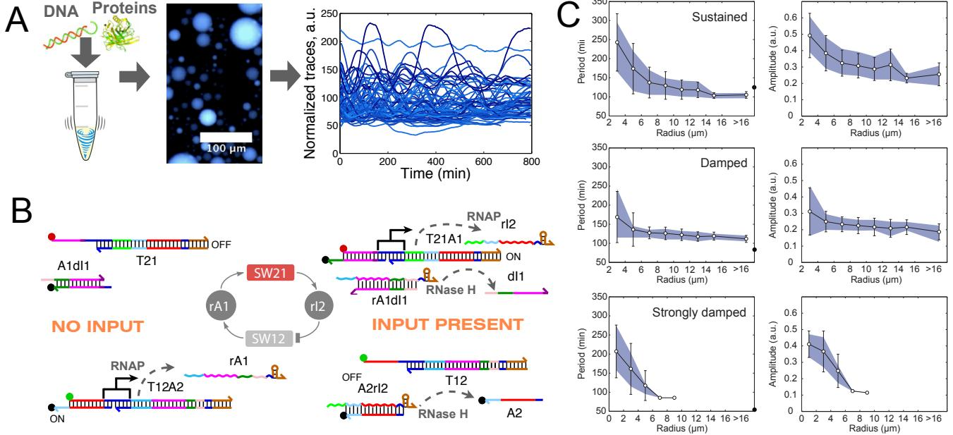
**Figure 1:** A: Scheme of our experimental method. B: Scheme of the compartmentalized oscillator [1, 4]. C: Period and amplitude diversity (for measured oscillatory traces only).
