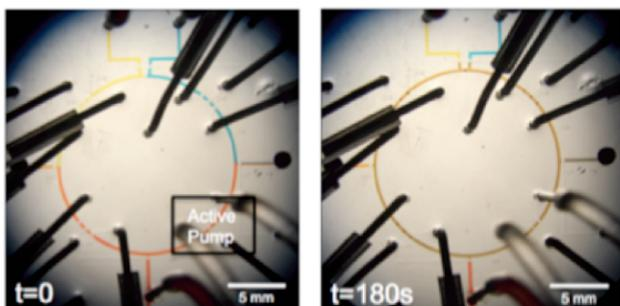
Figure 1. Mixing demonstration with food coloring in a microfluidic ring-mixer device.
