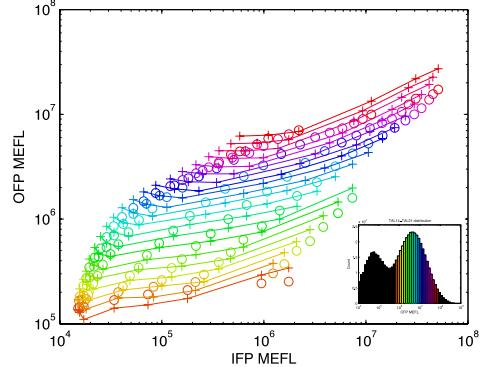
**Figure 2:** Experimental testing of two element cascades, such as this TAL14-TAL21 cascade, shows a good agreement between EQuIP predictions (circles) and observed experimental data (lines and crosses).
