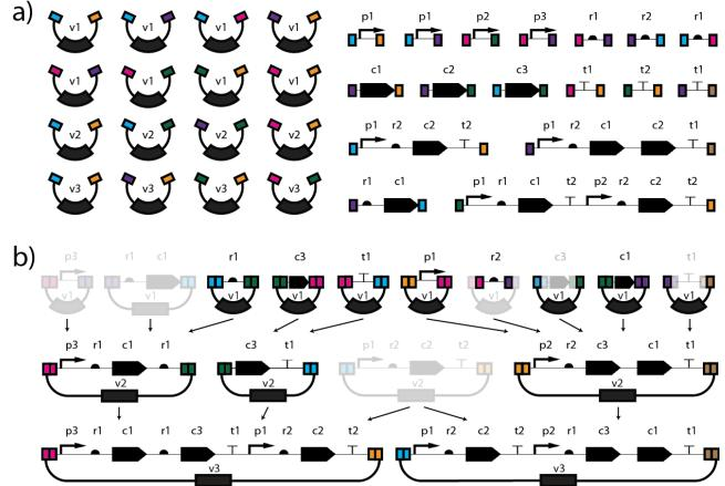
Figure 1: Example Optimized Assembly Plan a) Example existing library has a set of existing vector backbones, parts and devices with a variety of overhang pairs (shown as colored boxes) b) Example assembly plan re-uses parts and vectors from library (translucent) and shares intermediate parts. This assembly is performed in 2 stages, 6 steps and 13 PCRs.
