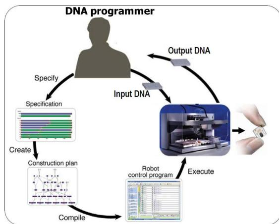
**Figure2. Overview of the CADMAD DNA editing technology workflow.** A biologist user specifies a library (top left). A construction plan is then computed and a robot control program for its execution is automatically generated (bottom). A robot/microfluidic device executes this plan (right) and its output is tested using one of the verification technologies we developed (1, 3, 4, 5).
