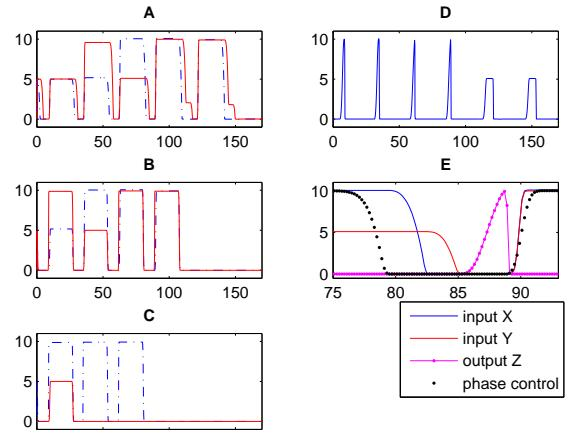
Figure 2: Simulation result: A. Waveforms for the two registers of  $r^0$ ; B. Waveforms for  $r^1$ ; C. Waveforms for  $r^2$ ; D. Waveform for  $Z = \text{NAND}(X, Y)$ ; E. Detailed waveforms in the range of 75 ~ 93 time units.
