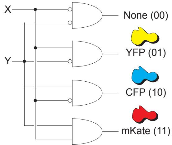
Figure 1: Boolean logic construction of a biological decoder with two inputs which are converted to fluorescent protein outputs.
